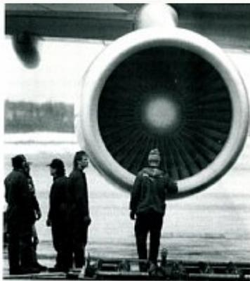
Figure 30. Crew examines one of the Boeing 747 jet engines that suffered extensive damage when the jet encountered an ash cloud on December 15, 1989. Copyrighted photograph by Bob Hamilton, Anchorage Daily News, reprinted by permission.
