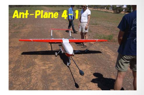
span: 2.6m, length: 2m, cruising to 600 km (max. 1108km, elevation 5800m), 86cc 2 cycle gasoline engine
